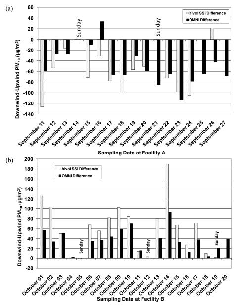
**Fig. 11.** Differences between downwind (Sites A-1 and B-1) and upwind (Sites A-2 and B-2) PM<sub>10</sub> concentrations for hivol SSI and minivol OMNI filter samplers at: a) Facility A during September 11–27, 2008, and b) Facility B during October 2–20, 2008.
