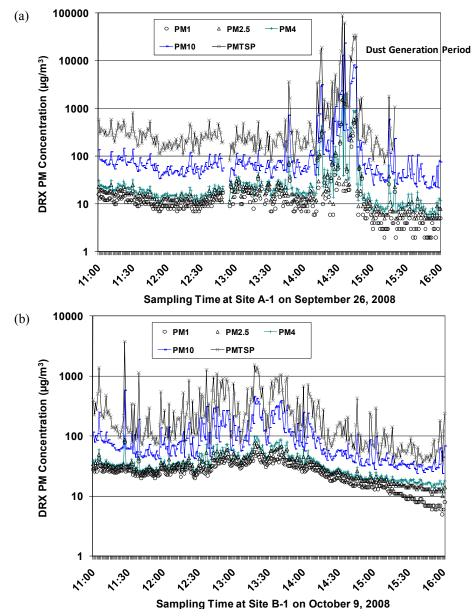
**Fig. 9.** One-minute DustTrak DRX size variations for days with the highest five-hour  $PM_{1.0}$  concentrations for: a) Site A-1 on September 26, 2008, and b) Site B-1 on October 9, 2008.
