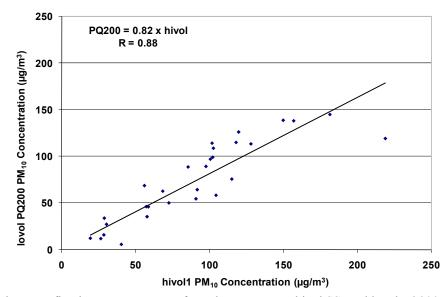
**Fig. 7.** Comparison between five-hour average  $PM_{10}$  from the two FRMs: hivol SSI and lovol PQ200 samplers at Sites A-1 and B-1. Samples during dust generation events at Site A-1 on September 25–26, 2008 are excluded.
