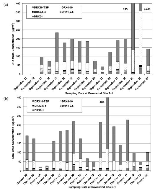
**Fig. 8.** DustTrak DRX mass size distributions at: a) Site A-1 during September 11–27, 2008, and b) Site B-1 during October 2–20, 2008. Particle size bins are in five size ranges:  $0-1 \mu m$ ,  $1-2.5 \mu m$ ,  $2.5-4 \mu m$ ,  $4-10 \mu m$ , and  $10 \mu m$ -TSP.
