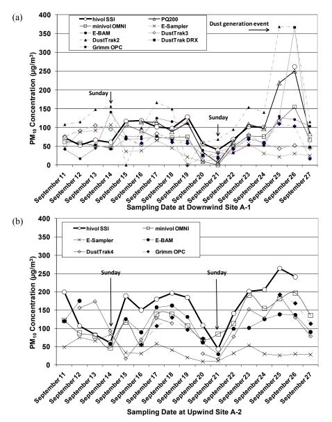
**Fig. 5.** Five-hour average  $PM_{10}$  concentrations for: a) downwind Site A-1, and b) upwind Site A-2 for the period from September 11–27, 2008. Fugitive dust events were simulated at Site A-1 during September 25–26, 2008 (Sundays were September 14 and 21, 2008).
