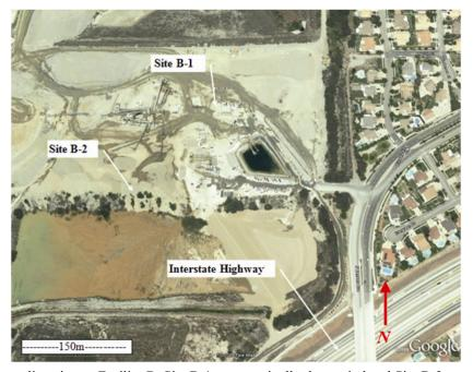
**Fig. 2.** Locations of sampling sites at Facility B. Site B-1 was nominally downwind and Site B-2 was nominally upwind of the sand and gravel operations (elevation 520 m above sea level [asl] for Site B-1 and 510 m asl for site B-2). Some roadway and storage pile configurations differed from those depicted in this satellite picture that was taken at an earlier date. Sampling at Facility B was conducted during October 2–20, 2008.
