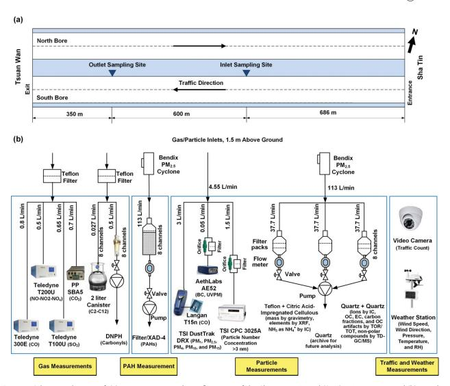
**Figure 1.** Schematic diagram of: (a) west section sample configuration of the Shing Mun Tunnel (SMT) in Hong Kong and (b) sampling setup at the outlet site of the SMT in 2015.
