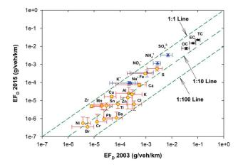
**Figure 4.** Comparison of  $PM_{2.5}$  elements (circle), ions (triangle), and carbon (star) emission rates measured in 2003 and 2015. Error bars represent standard error of the mean.
