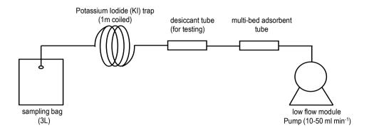
Figure 1. Schematic of the sampling system for laboratory performance test.
