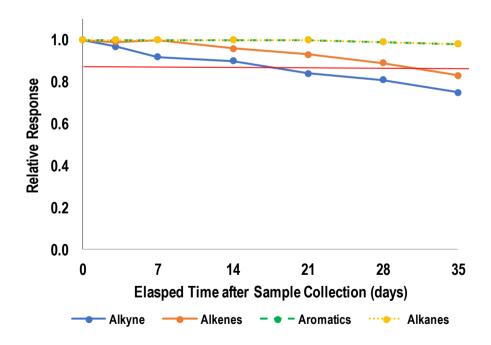
Figure 3. Relative responses of VOCspams collected on the adsorbent tubes stored at 0 and  $10^{\circ}$ C for the duration of 35 days (the red line represents the relative responses at 90%).
