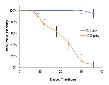
Figure 4. Efficiencies of ozone removal for a laboratory-made potassium iodide coated copper tube for O<sub>3</sub> concentrations of 200 and 1000 ppb.
