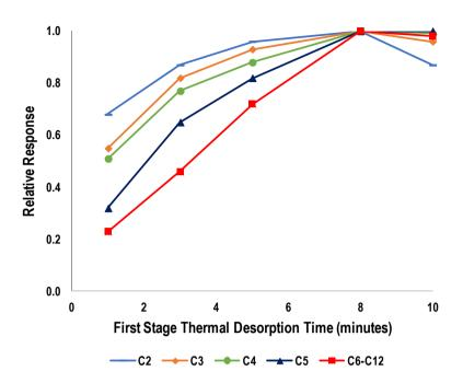
Figure 6. Relative responses of  $VOC_{SPAMS}$  desorbed from the adsorbent tubes loaded with standard at 330°C in the first stage of thermal desorption for 1-10 minutes.
