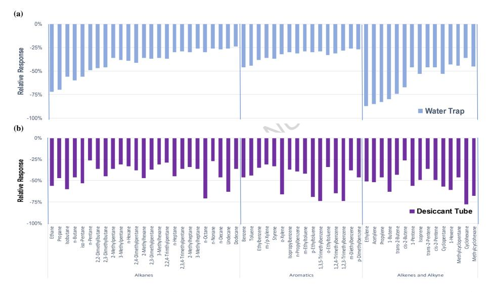
Figure 5. Relative responses for the target VOCs using two types of dyes: a) water tap and b) desiccant tube dryers with calcium sulfate (CaSO<sub>4</sub>). Samples are normalized to measurements without proceeding dryers.
