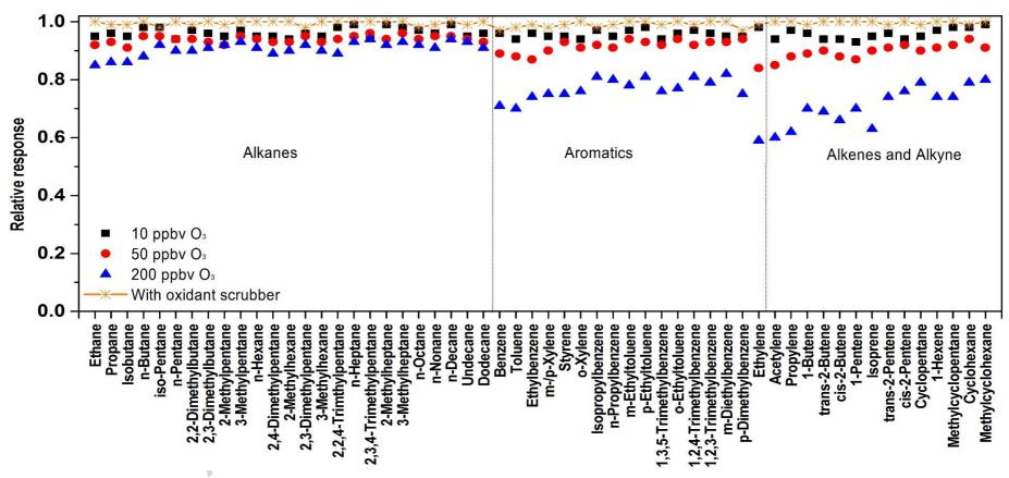
Figure 2. Relative responses of the 57 VOCs collected at ozone concentrations of 10, 50, and 200 ppbv. Relative response with O<sub>3</sub> scrubber is also shown for comparison.
