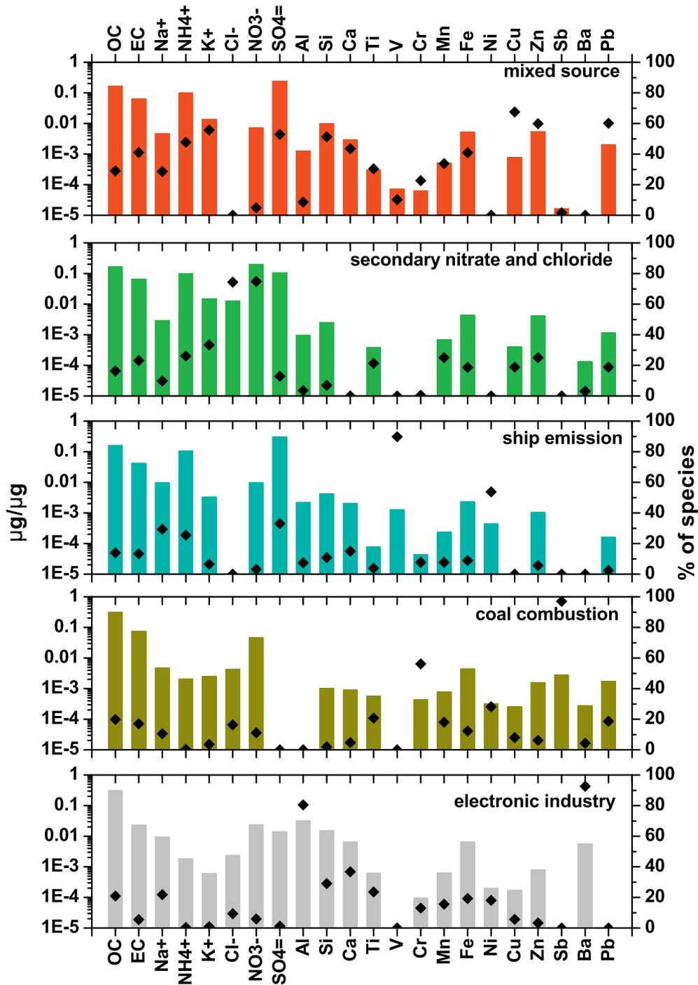
Fig. 6. Five source profiles (bars and left y-axis) and percentage contributions (dots and right y-axis) of each chemical component resolved from PMF model analysis in suburban Zhuhai.
