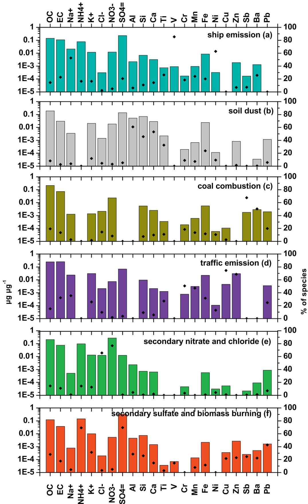
Fig. 3. Six source profiles (bars and left y-axis) and percentage contributions (dots and right y-axis) of each chemical component resolved from PMF model analysis in urban Guangzhou.
