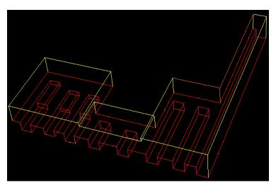
Fig. 2. Grid generated by Gambit in five parts.
